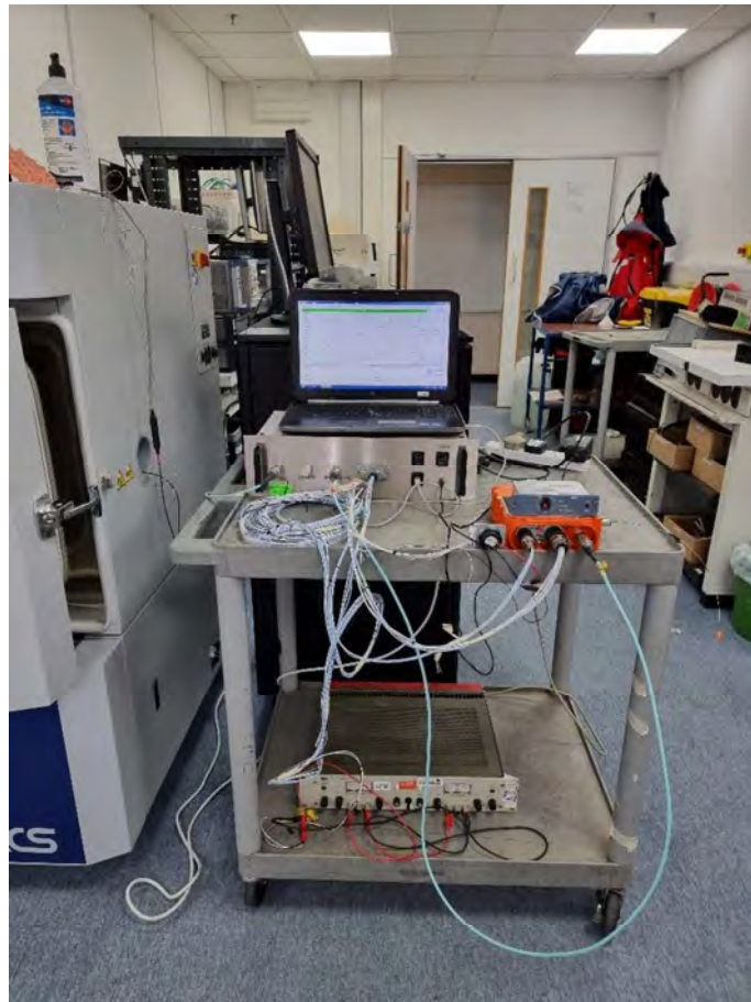
Test Configuration for Conducted RF Tests
