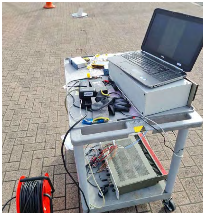
Satellite Qualitative Test and Acquisition Time and Position Accuracy Test (A.3.8.2.1) – Configuration 6
