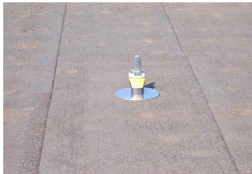
Configuration 7: Beacon on ground plane
