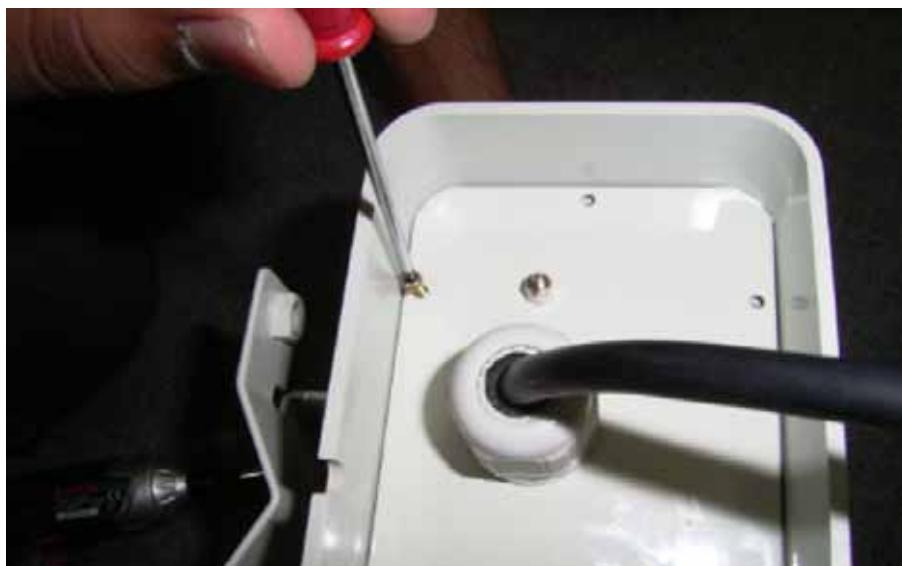
If You use the External Antenna. The Antenna cable connects with a WA500-SU N-type Connector.
