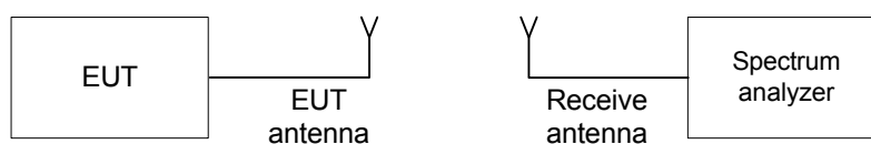
Figure 7.2.1 Occupied bandwidth test setup
