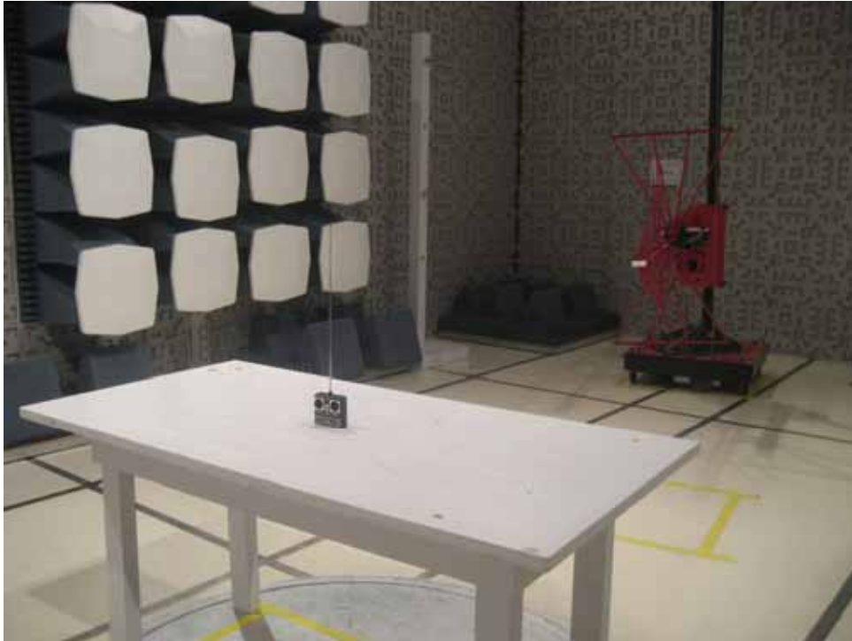
RADIATED EMISSION TEST SETUP
