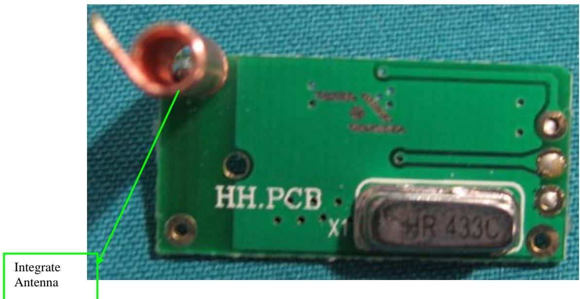
***Integrate Antenna without Connector View***
