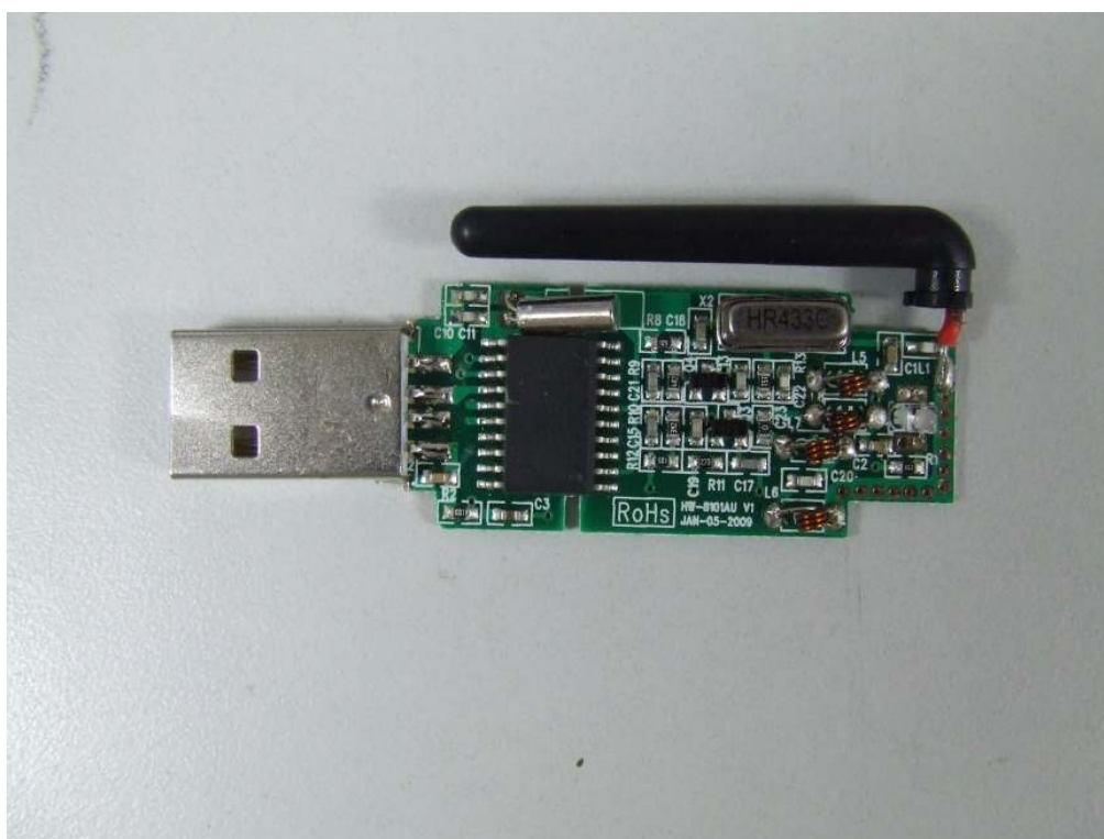
Photo 2-Front view of RF Main Board
