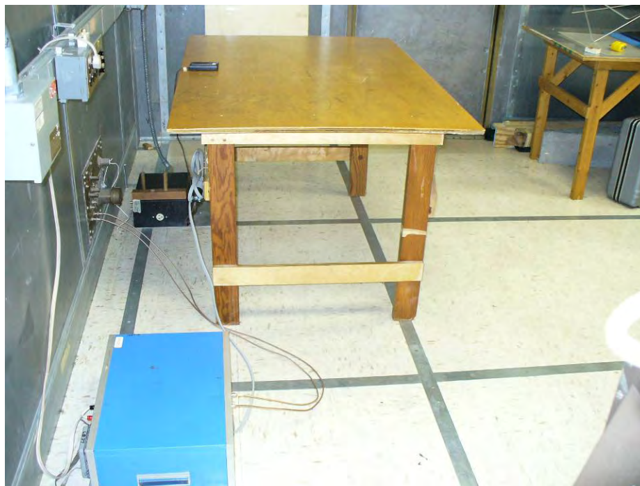
Photographs 1 & 2: Conducted Emission Setup
