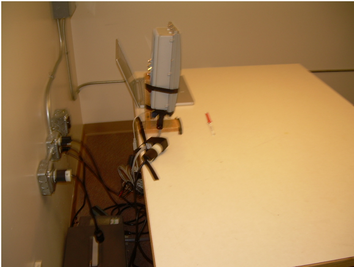
Photograph 4 - Back View Conducted Disturbance Worst Case Configuration
