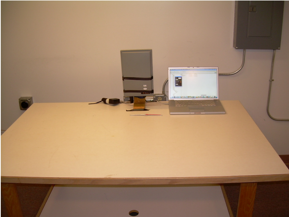
Photograph 3 - Front View Conducted Disturbance Worst Case Configuration
