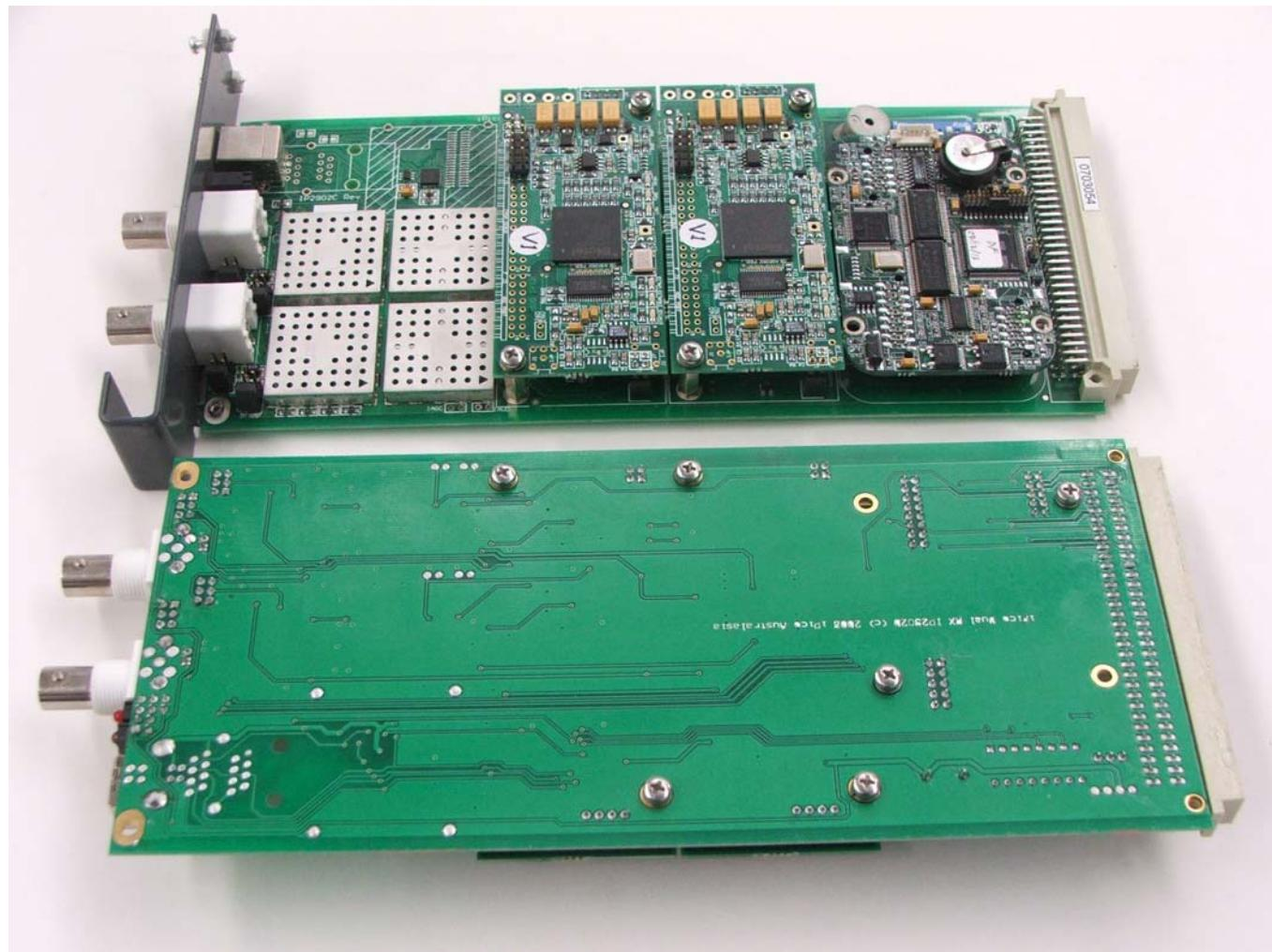
Dual channel TRF receiver section located under metal shields.
