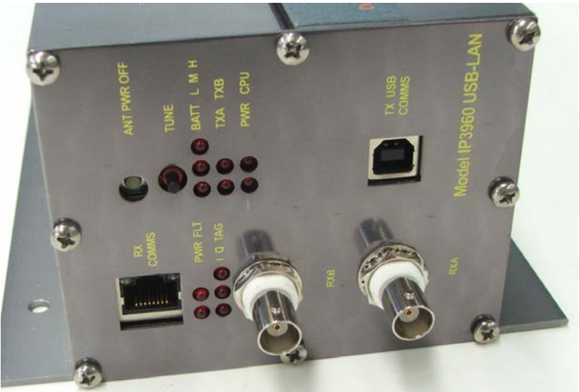
Front Panel with RX antenna connectors and Diagnostic LEDs
