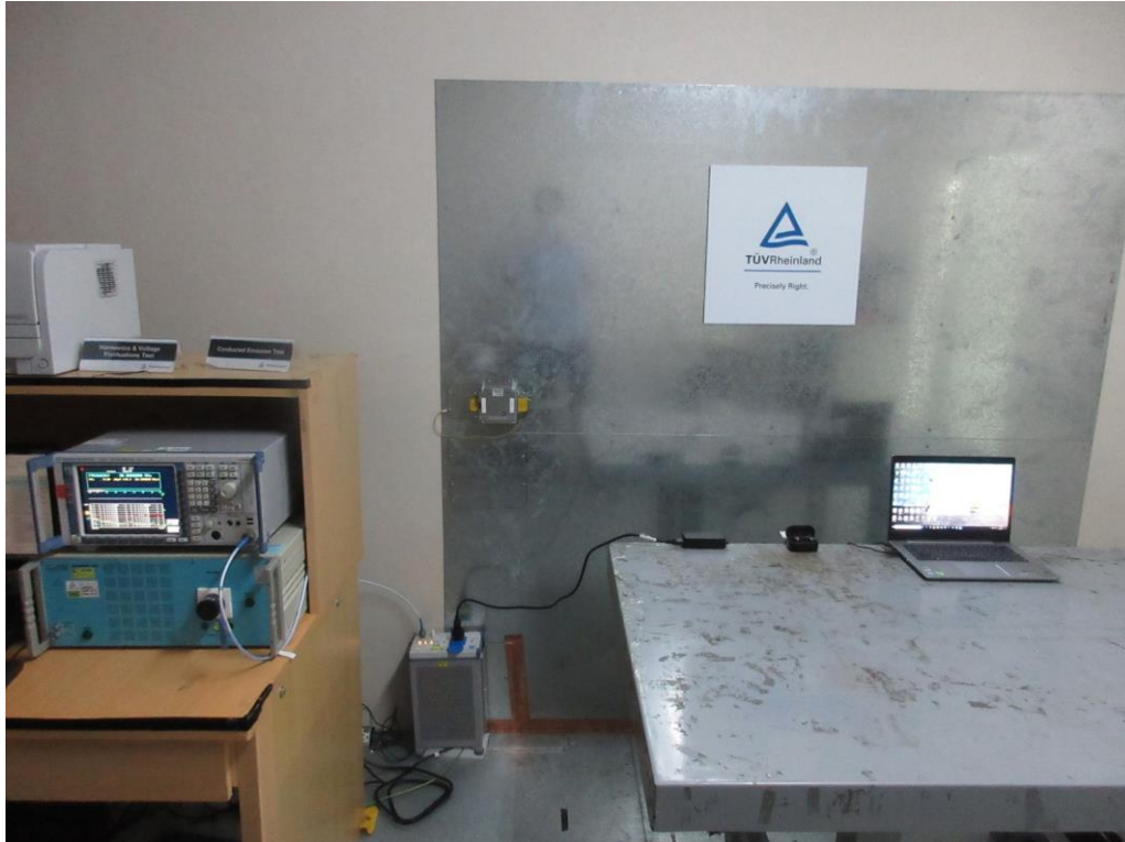
Photograph 15: Set-up for AC Mains (Front View)
