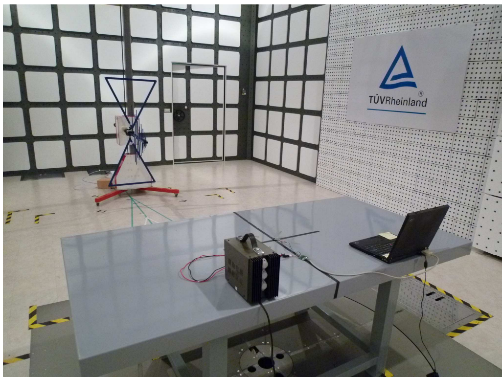
Photograph 2: Set-up for Spurious Emissions (Back View 1)
