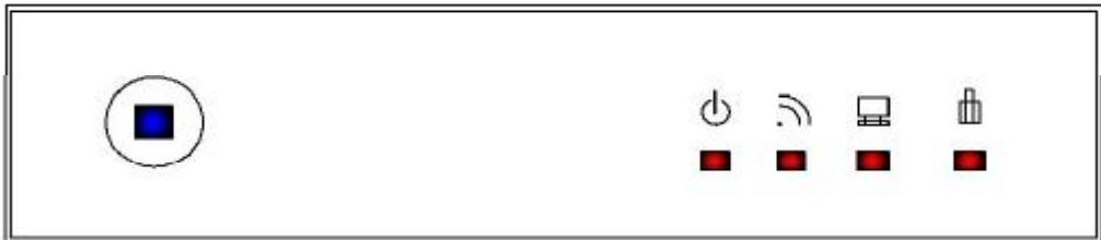
**POWER(Yellow):** A solid light indicates a proper connection to the power supply.
