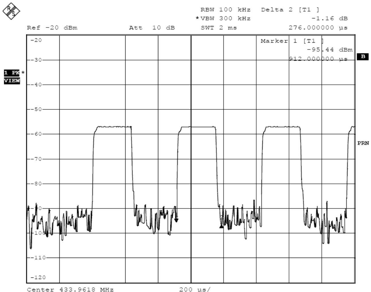
The graph shows the duration of short 'on' signal. From marker 1 to marker 2, duration is 0.276ms.
