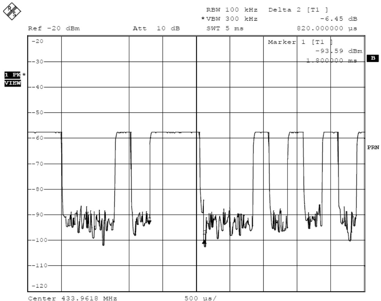
The graph shows the duration of middle 'on' signal. From marker 1 to marker 2, duration is 0.82ms.
