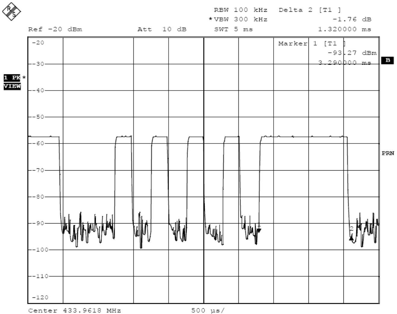
The graph shows the duration of long 'on' signal. From marker 1 to marker 2, duration is 1.32ms.
