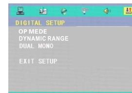
DYNAMIC RANGE: When "LINE OUT" is selected, choose this setting to adjust the line out ratio and get different effect. If set to FULL, the audio signal peak value will be the minimum. If set to OFF, signal peak value will be the maximum.
