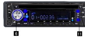
11. **Time Displaying:** Press **11** (DSP) button and the current time is displayed, and it returns to original status after 5 seconds or press. The button again.
