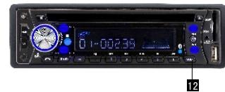
12. Press **12** (MOD) button to select radio mode, playback mode or audio in mode.
