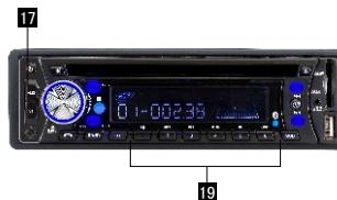
5. Press **17** (AMS) button to scan each stored station 10 seconds respectively which stored in **19** (1~6) number buttons. When AMS mode is carried out. "INT" appears on display. (See the picture). You also can press the corresponding number button or AMS button when your desired station is charged. It starts playing that station.
