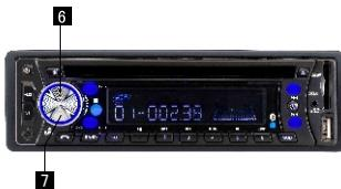
6. You can adjust the sound level by rotating the **6** (VOL) knob.
