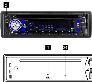
1. Operating the unit for the first time or after replacing the car battery, you must reset the unit. Press 1 (RES) button with a pointed object (such as a ballpoint pen) to set the unit to initial procedure.
