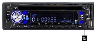
2、Press **15** ( **▶** or **◀** ) to choose your favorite track upward or downward respectively. Press and hold **15** ( **▶** or **◀** ) button to fast forward or rewind the track upward or downward respectively.
