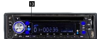
13. Receptor for the card remote commander. (For remote control version only)
