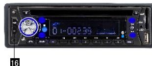
3. press **16** (ST) button to select mono mode or stereo mode. Stereo reception is charged when "ST" appears in the LCD and "◎◎" appears in the display.
