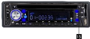
2. **Manual Tuning:** press **15** (► or ◄) button continuously to select a station upward or downward respectively. **Automatic Tuning:** Press and hold **15** (► or ◄) button for more than 3 seconds, the radio automatically search a station upward or downward respectively and plays when it find a station.
