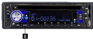
7. Press **8** (LOU) button to increase the low frequency. This can improve the sensitivity for your ears, And “LOUD” appears in the LCD when the loudness mode is activated.
