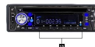
4. During playback, press “**INT**” button, one of the number button **19** to play the first 10 seconds of each track on the disc, the display will show “**INT**, track number and elapsed time” ( See the picture ), which indicates **INT** function is already activated.
