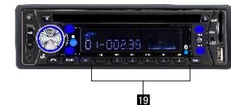
6. During playback, press **19** “**PAUSE**” button to suspend the playback, “**PAUSE**” mark stops running in the display. To return to normal play mode, press it again, and “**PAUSE**” mark runs accordingly.
