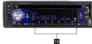
5. During playback, press **19** “**RDM**” button, and “**RDM**” appears on the display (See the picture), which indicates **RDM** function is carried out. The unit plays any track at random. Press **RDM** once more to return to normal playback mode.
