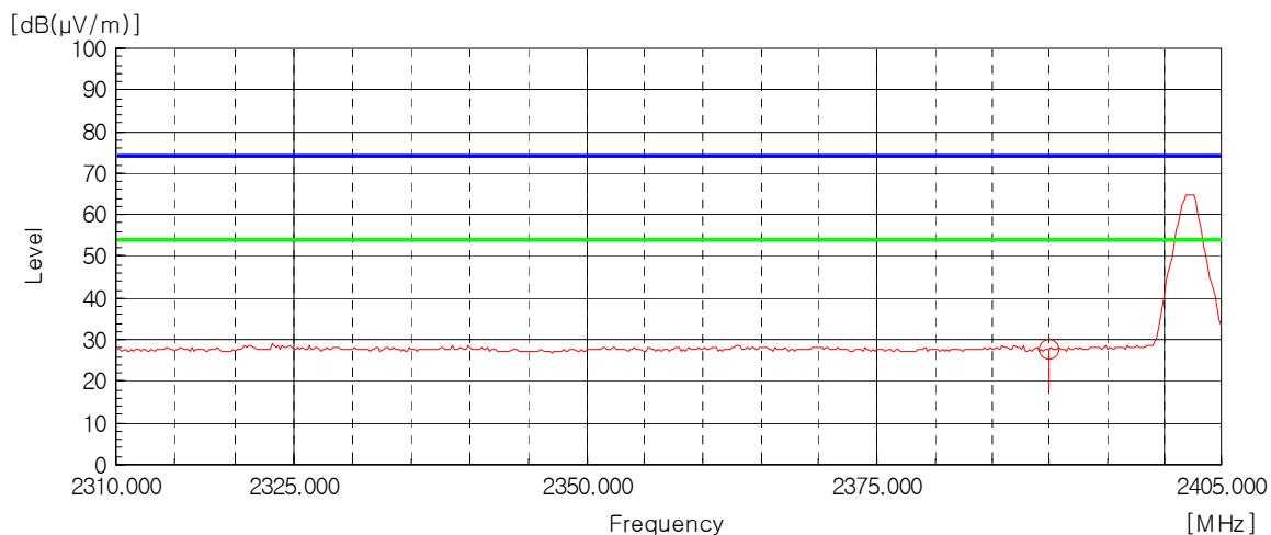
Peak Detector: RBW: 1 MHz, VBW: 1 MHz (2 483.5 MHz - 2 500.0 MHz), Worst case (High, Vertical)
