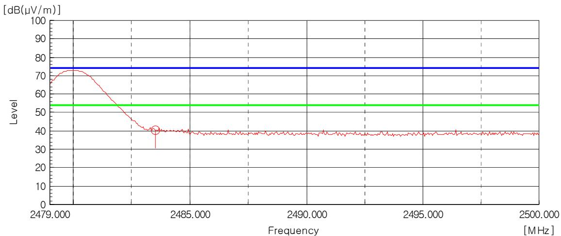
AV Detector: RBW: 1 MHz, VBW: 10 Hz (2 483.5 MHz - 2 500.0 MHz), Worst case (High, Vertical)
