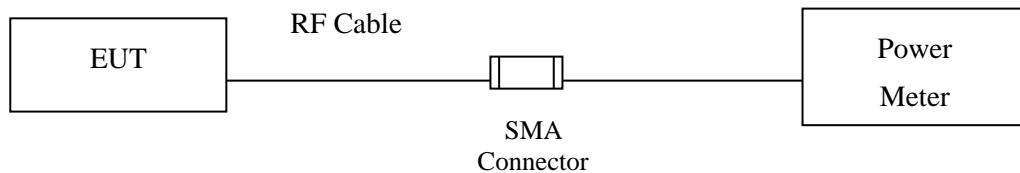
Conduction Power Measurement (for 802.11ac)
