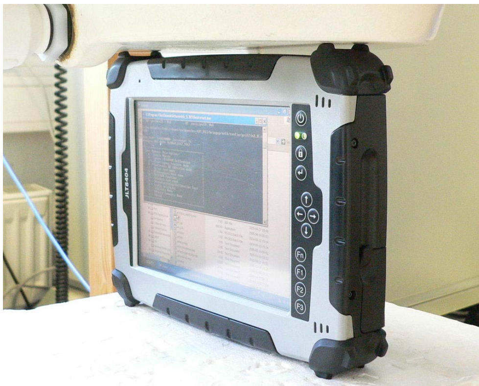
Fig. 19: Tested position for Antenna B, upper edge touching the phantom.
