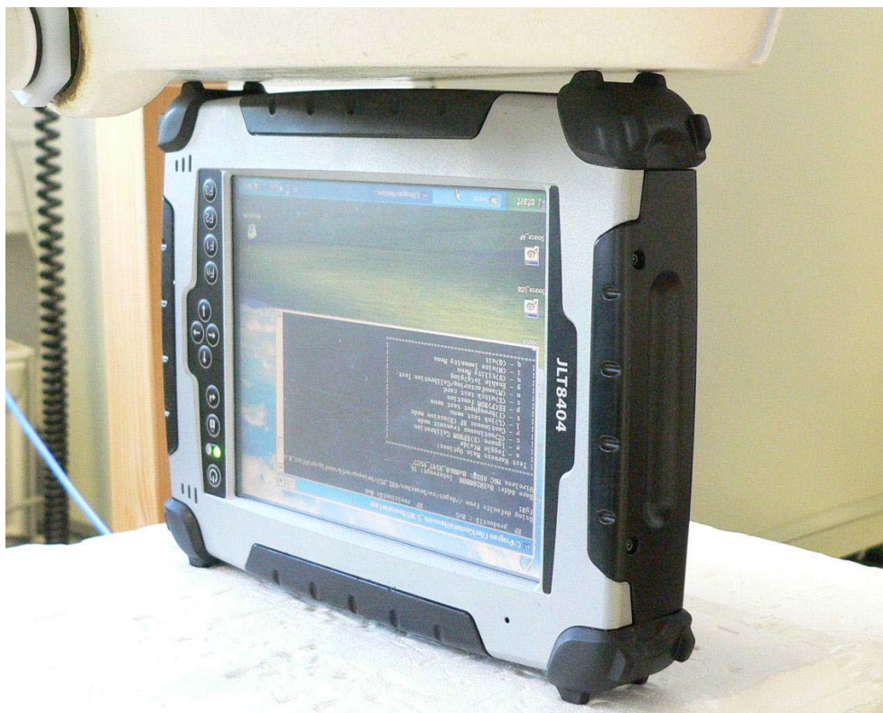
Fig. 21: Tested position for Antenna A, bottom edge touching the phantom.
