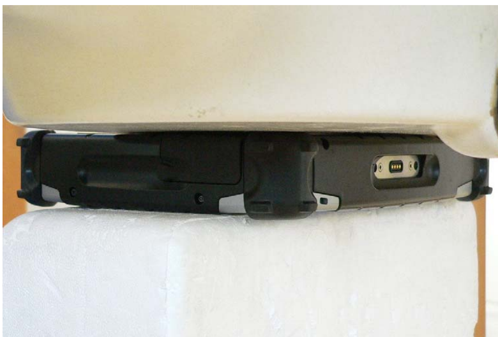
Fig. 22: Tested position for Antenna A, lap held position.
