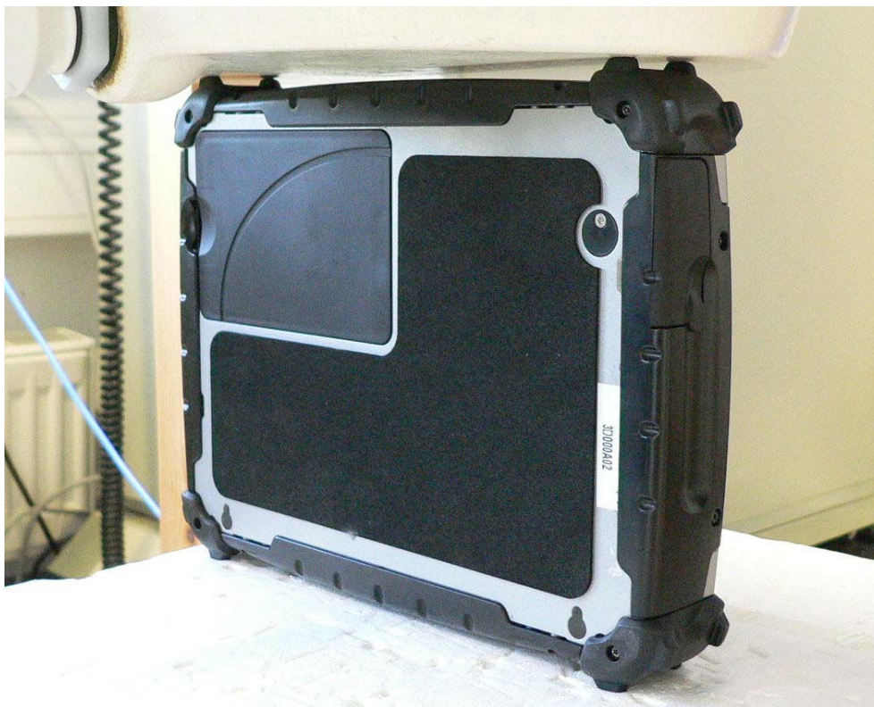
Fig. 17: Tested position for Bluetooth Antenna, bottom edge touching the phantom.
