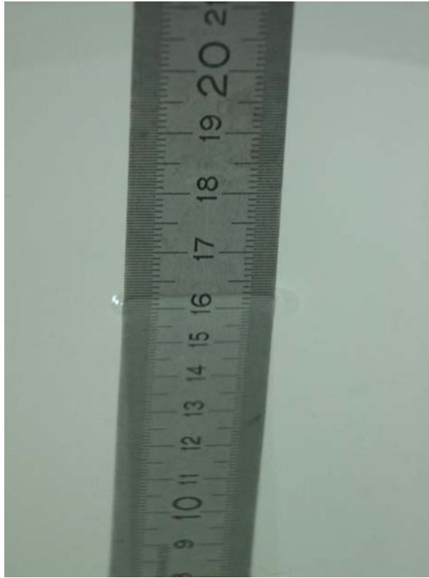
Fig. 23: Liquid depth for 2450 MHz Body measurements.
