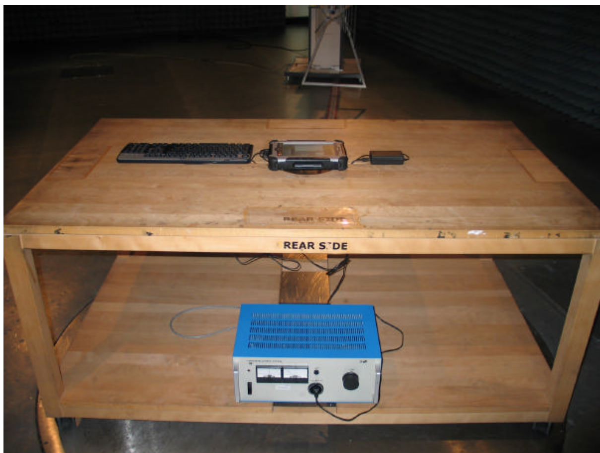
Photo 2: Test setup for radiated measurements
