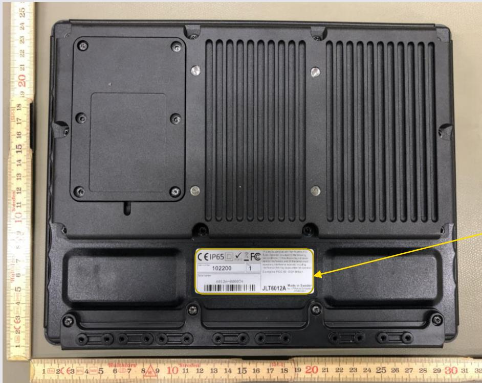
Thermal Transfer Polyester Label by 3M with thermal inc
