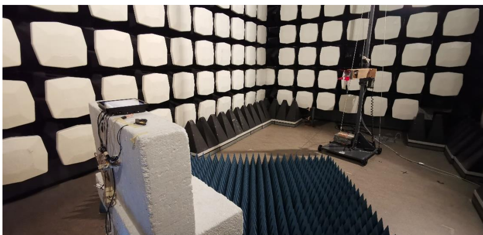
Photo 4. Test set up 1 – 18 GHz.
