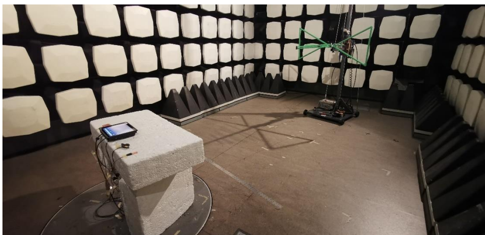
Photo 3. Test set up 30 – 1000 MHz.
