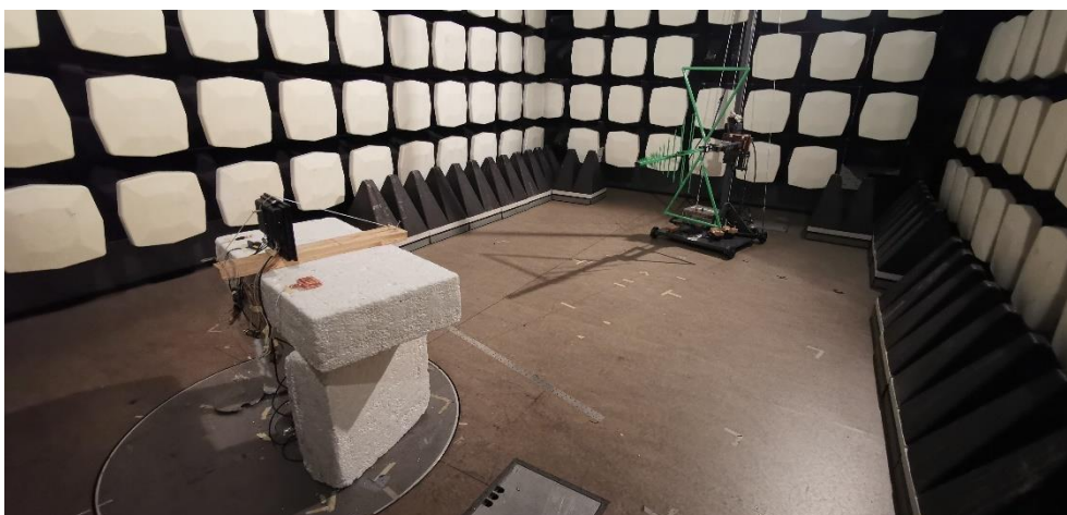
Photo 7. Radiated emission test setup in SAC. 30 - 1000 MHz. EUT vertical.
