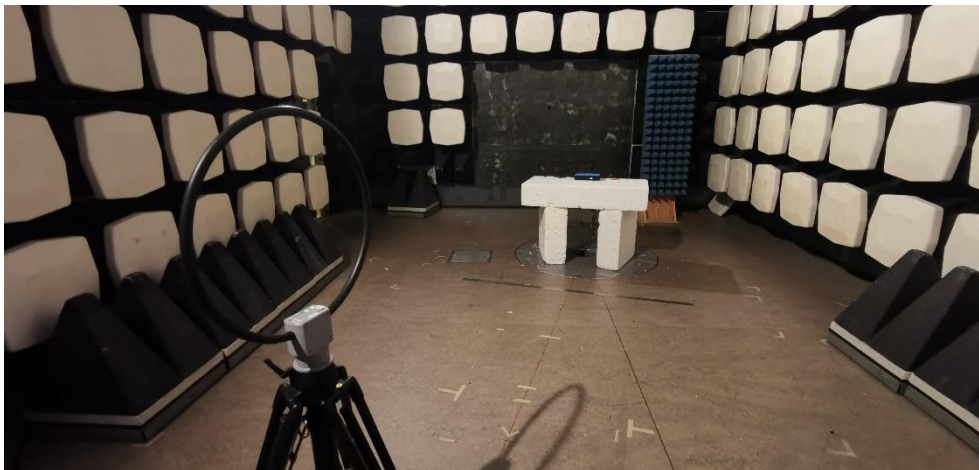
Photo 6. Radiated emission test setup in SAC. 9 kHz – 30 MHz. EUT horizontal.
