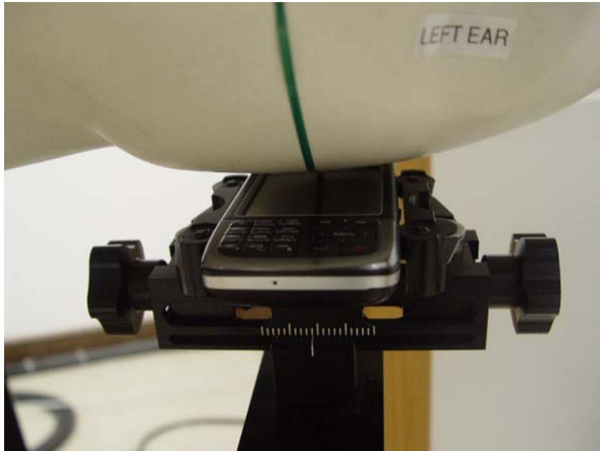
SAR Test Setup (Device at Head Phantom) – Closer Front View (Ear/Tilt)
