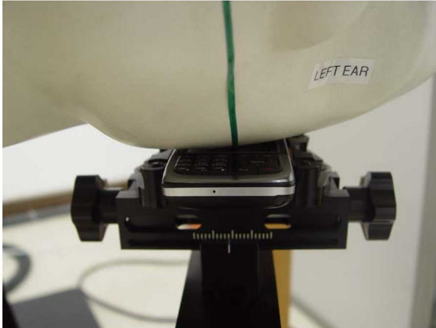
SAR Test Setup (Device at Head Phantom) – Closer Front View ( Cheek/Touch )
