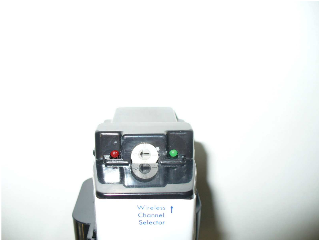
Fig. 4: Camera front view (channel selector and power led detail)
