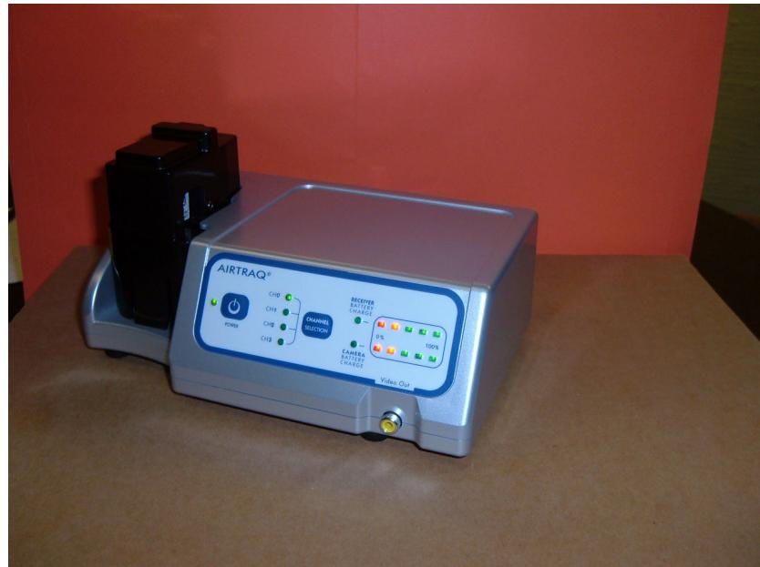
Insert the camera on its slot. The camera will automatically start charging its battery.
