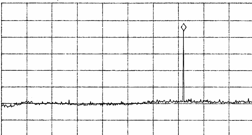
Figure four Peak Radiated Emissions taken at 1 meter in screen room.
