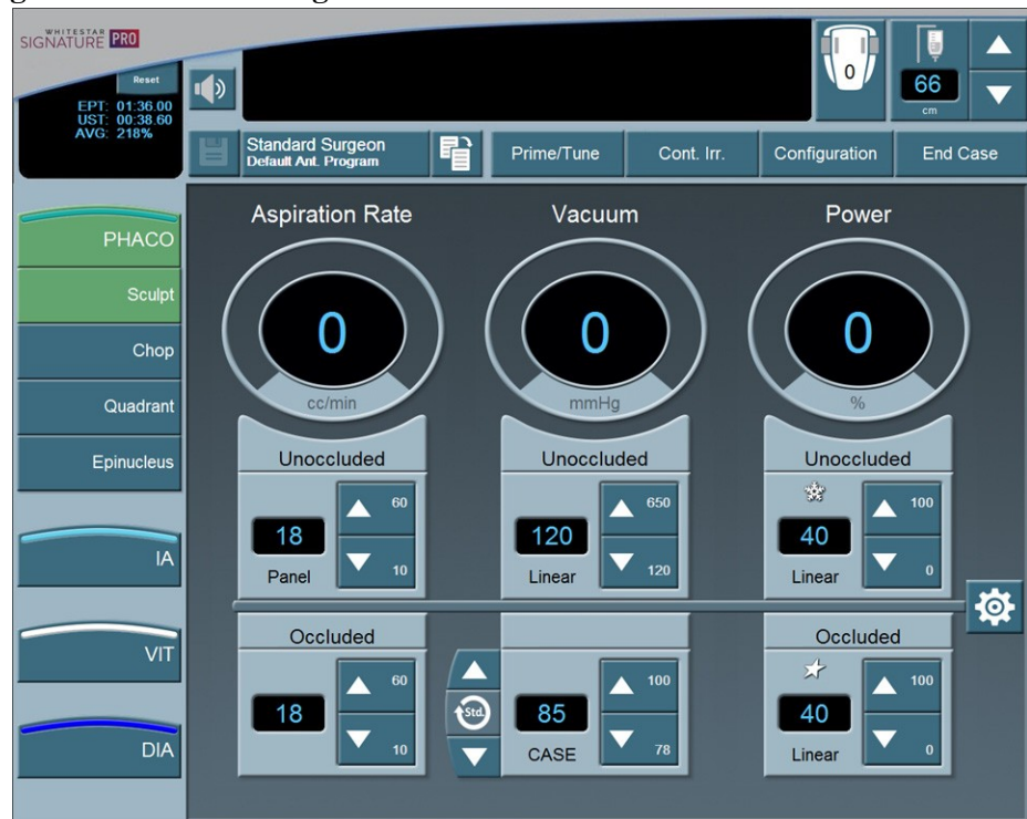
Figure 5.14 – Phaco Surgical Screen with Occlusion and CASE On
