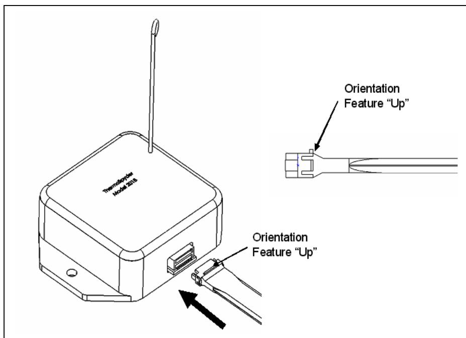
**TIP:** To make network initialization easier, install the ThermoProbe or ThermoAdapter / thermocouple assembly before starting to test. During network initialization, DataLink checks for open thermocouples so having the thermocouples connected to the ThermoSpyder speeds the initialization step.
