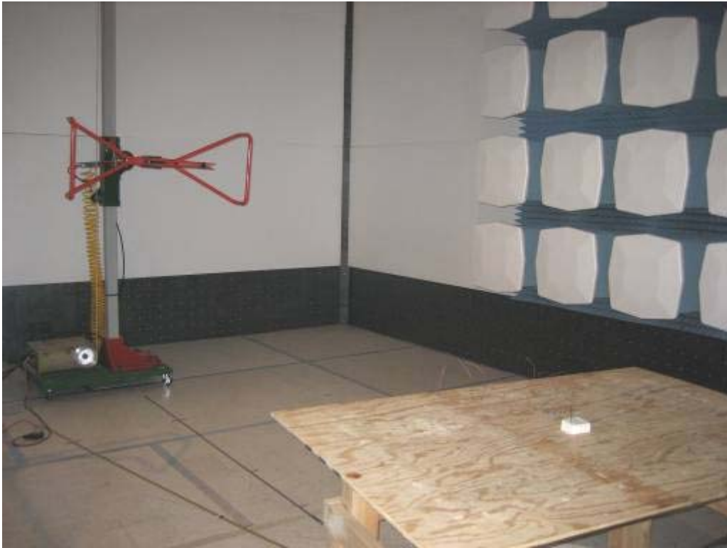
Radiated Emission Setup View
