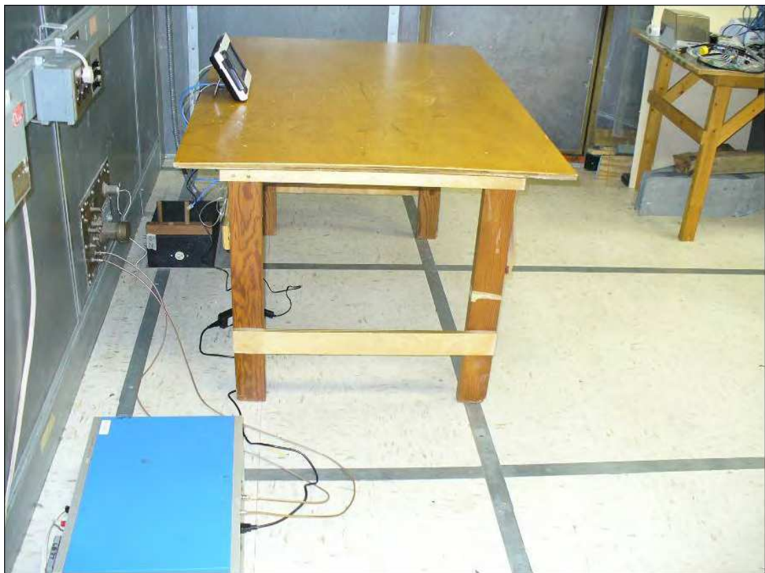
Conducted Emission Setup
