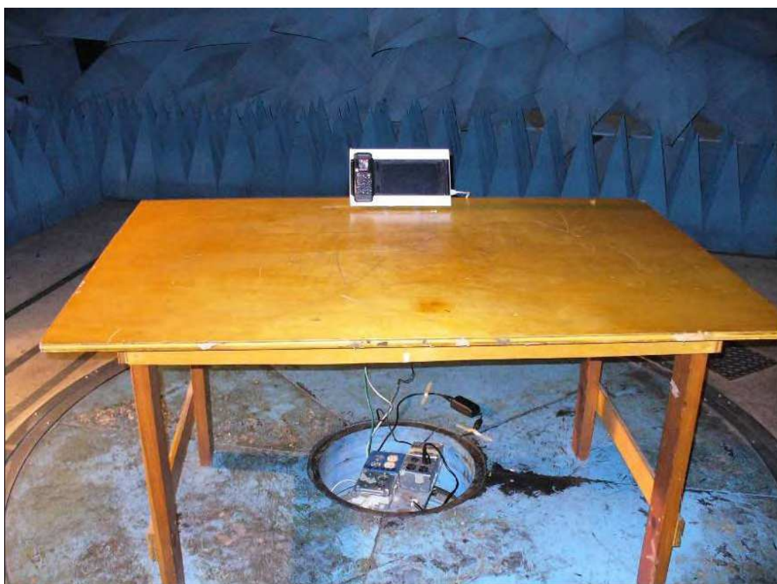
Radiated Emission Setup
