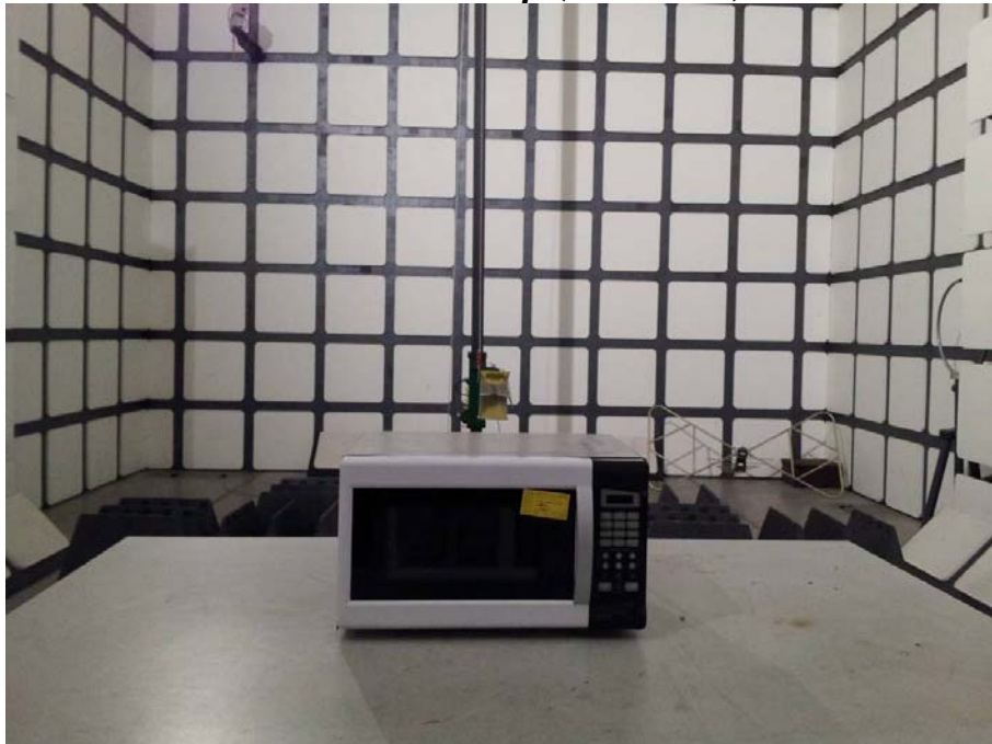
Radiated Emission Test Set-up (1~25GHz) :
