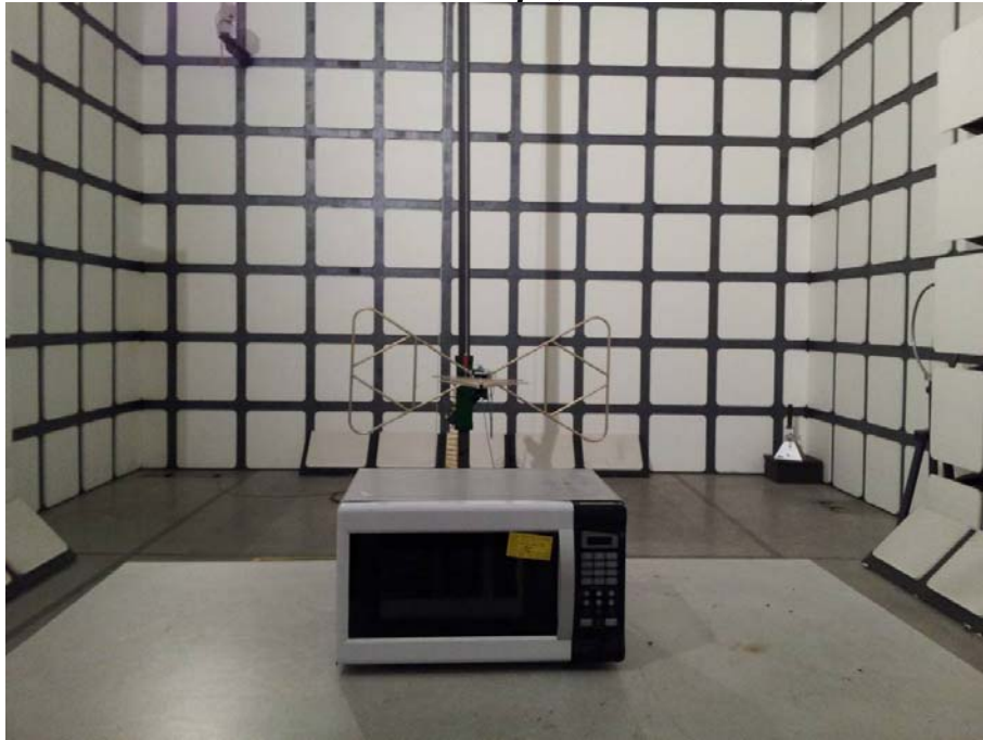
Radiated Emission Test Set-up (30~1000MHz):
