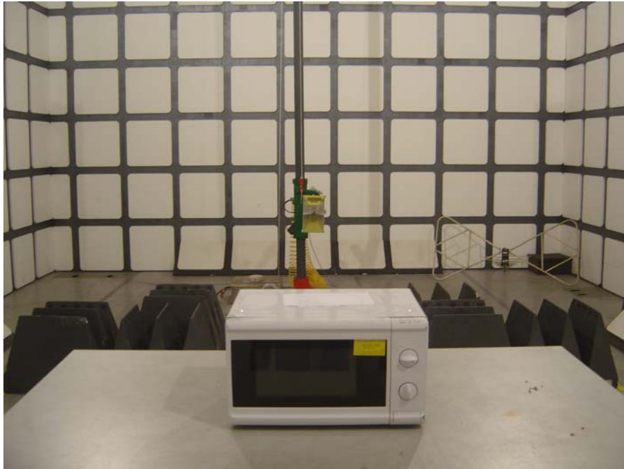
Radiated Emission Test Set-up (1~25GHz):
