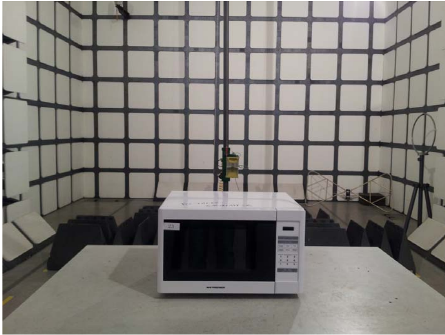
Operating Frequency Test Set-up
