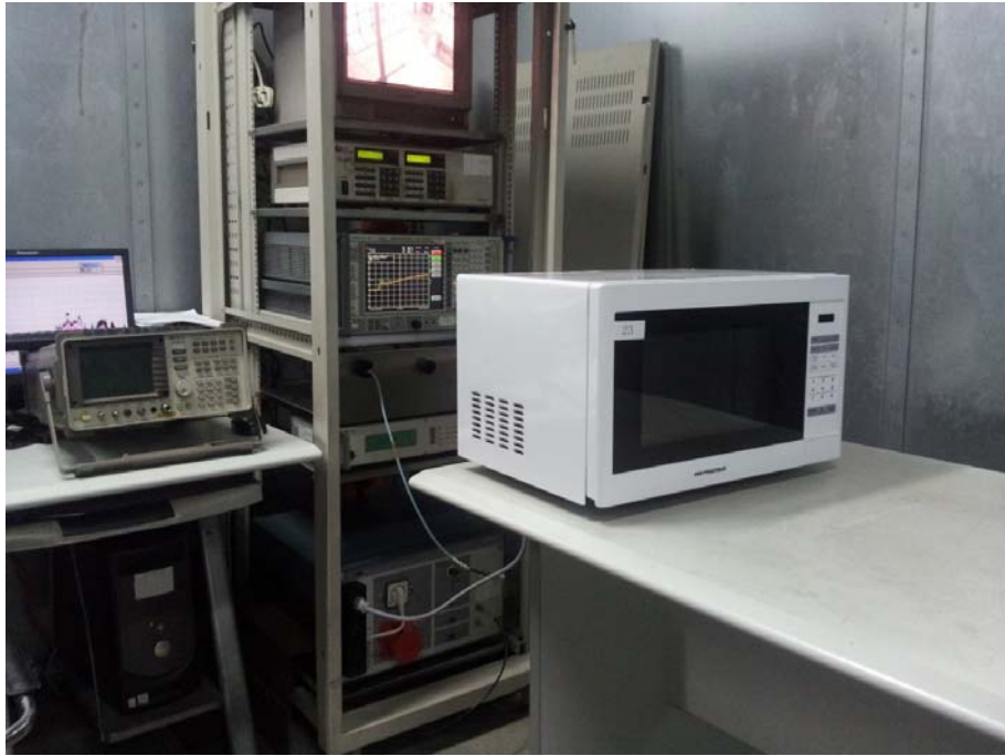
Conducted Emission Test Set-up
