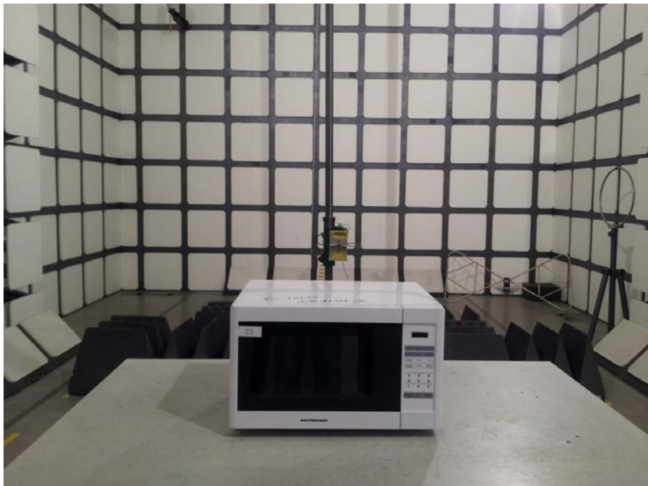
Radiated Emission Test Set-up (1-25GHz)
