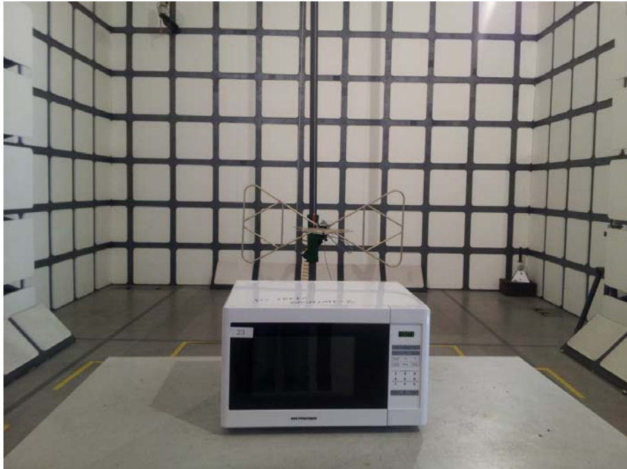
Radiated Emission Test Set-up (30 -1,000MHz)
