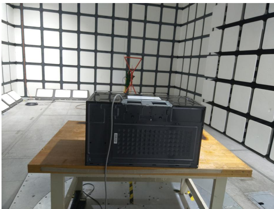
Radiated Emissions - Rear View (30 MHz – 1 GHz)
