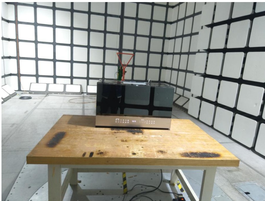
Radiated Emissions - Front View (30 MHz – 1 GHz)
