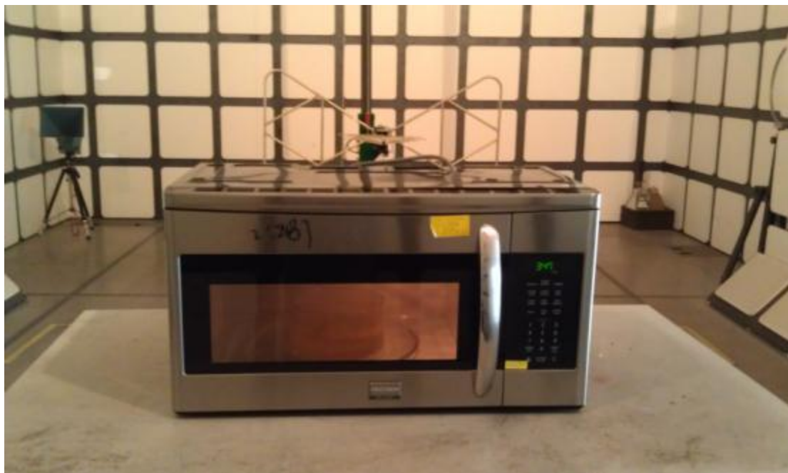
Radiated Emission Test Set-up (30 -1,000MHz)
