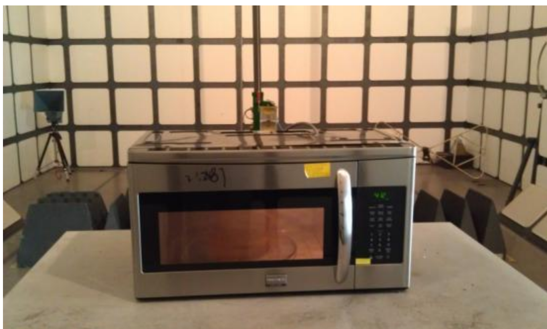
Radiated Emission Test Set-up (1-25GHz):
