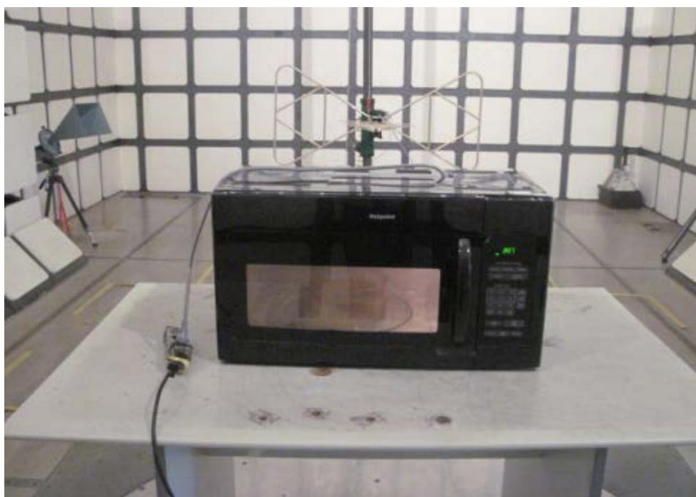
***Radiated Emission Test Set-up (1-25GHz):***
