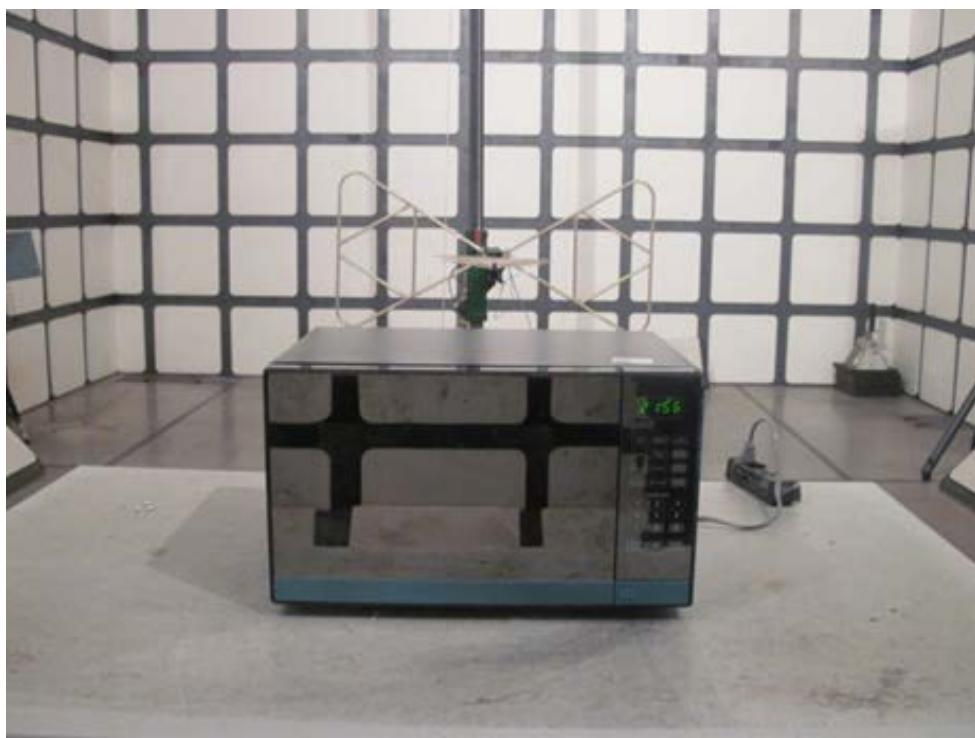
***Radiated Emission Test Set-up (1-25GHz):***
