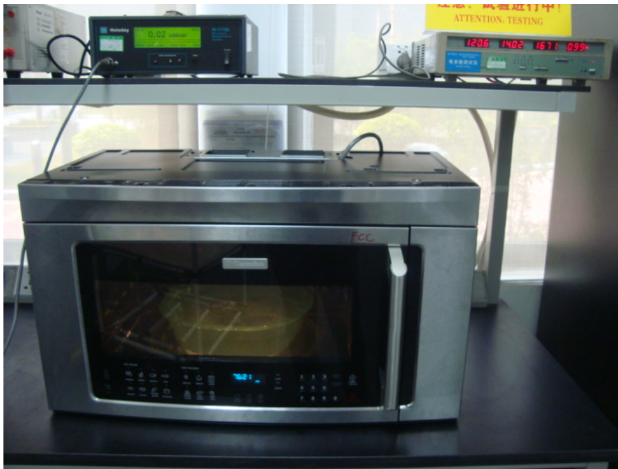
Radiation Hazard Test Set-up
