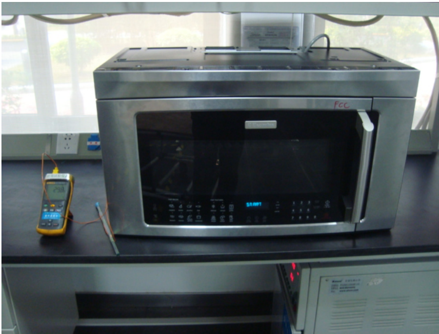
RF Output Power Test Set-Up
