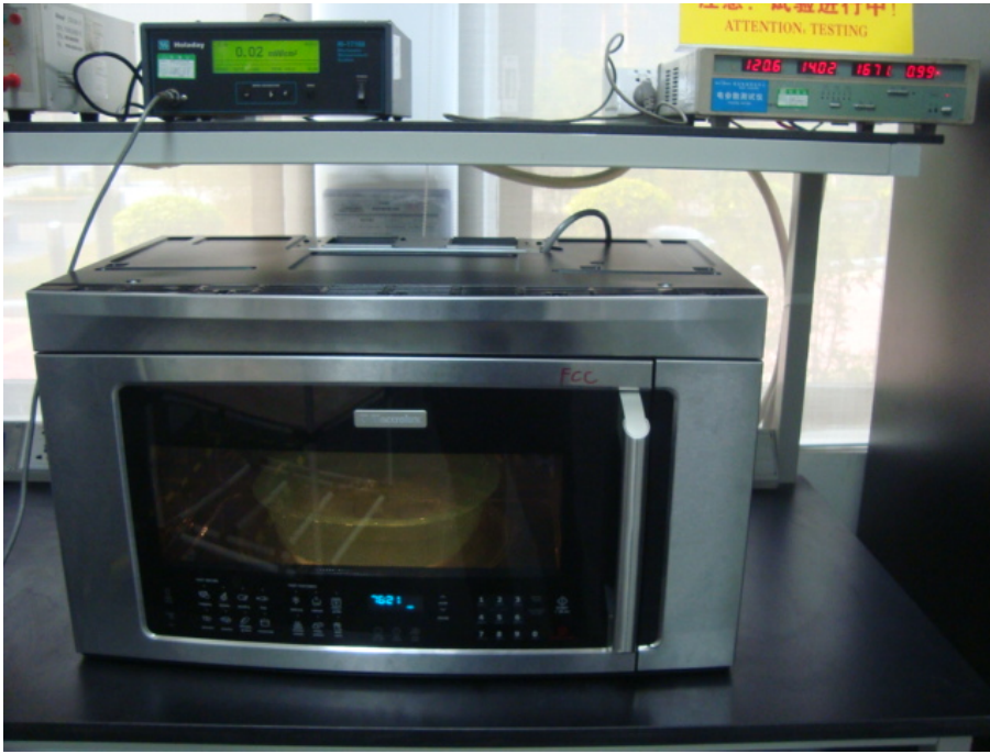
Input Power Test Set-Up
