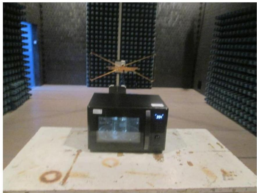
**2. Radiated Emission Measurement above 1GHz**
