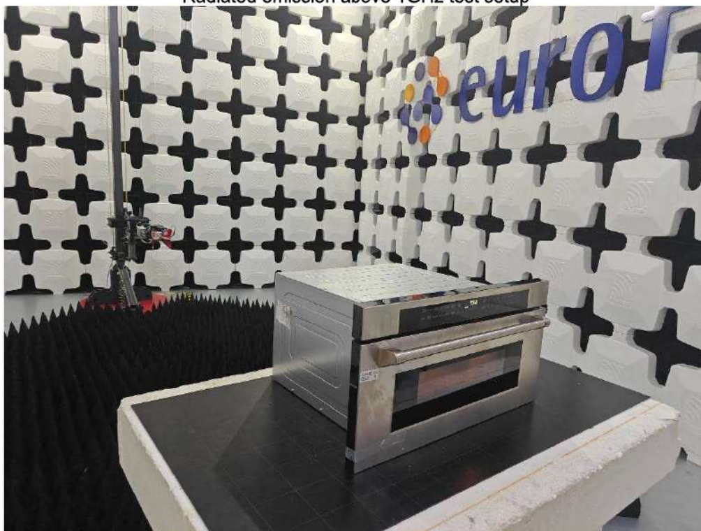
Radiated emission above 1GHz test setup
