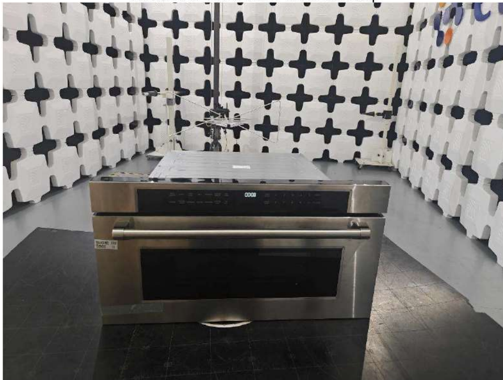
Radiated emission above 1GHz test setup
