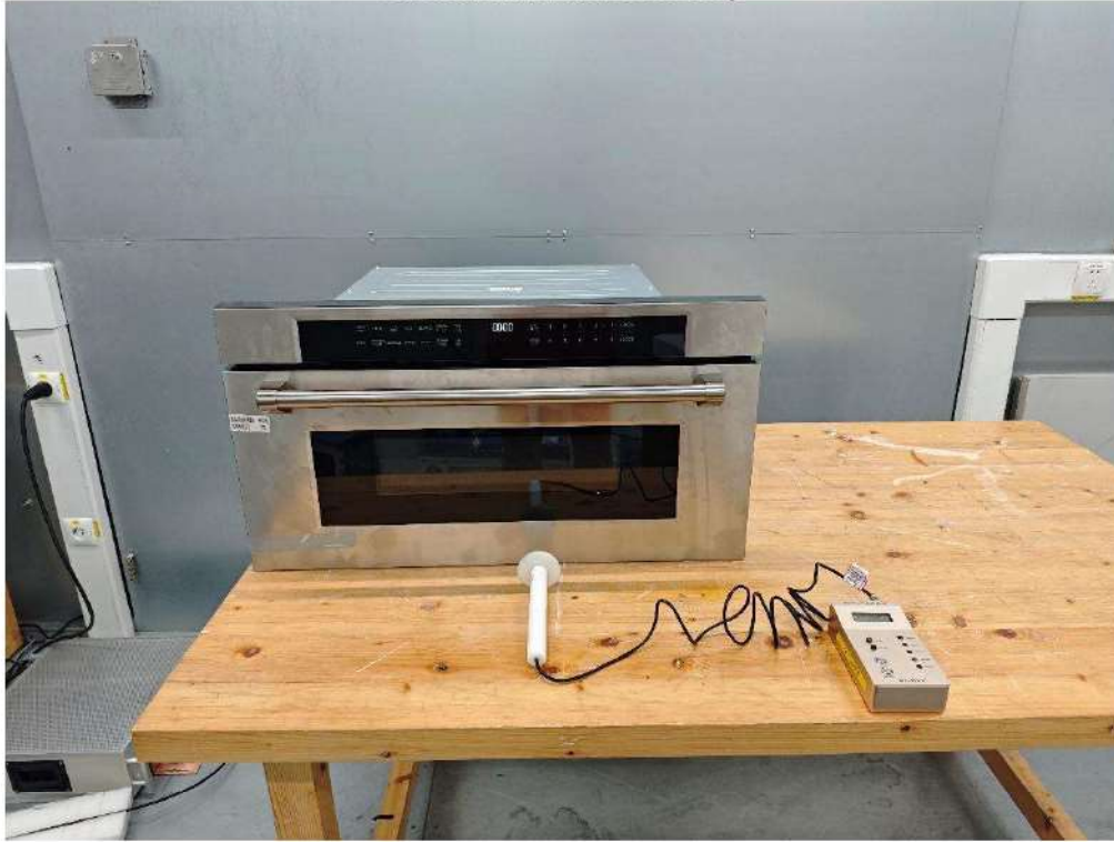
Radiation hazard test setup
