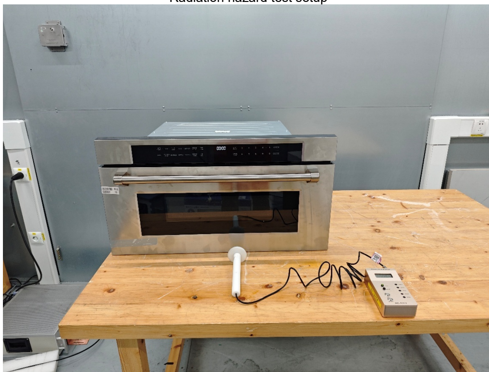
Radiation hazard test setup
