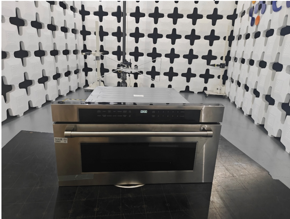
Radiated emission above 1GHz test setup
