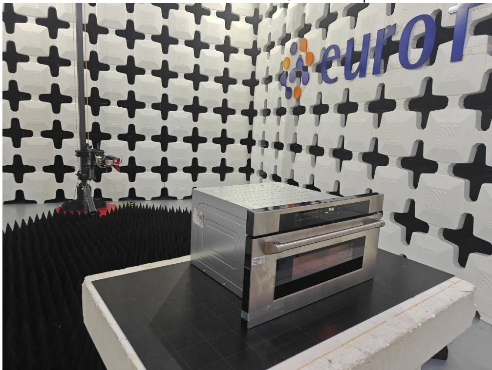
Radiated emission above 1GHz test setup
