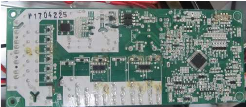
new power board-bottom view
