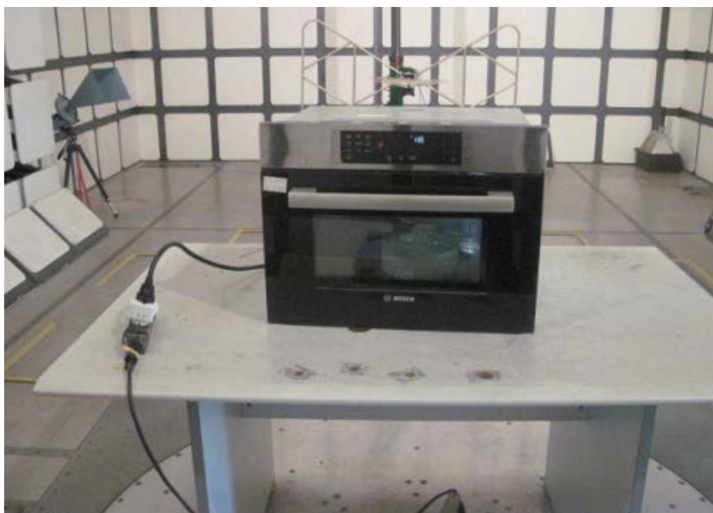
***Radiated Emission Test Set-up (1-25GHz):***
