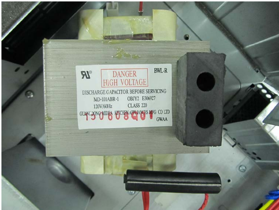
High-voltage Transformer View
