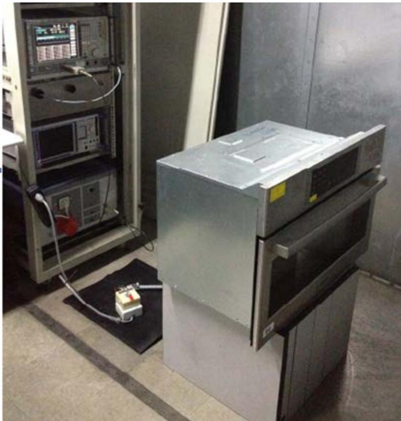
***Radiated Emission Test Set-up (30 -1,000MHz):***
