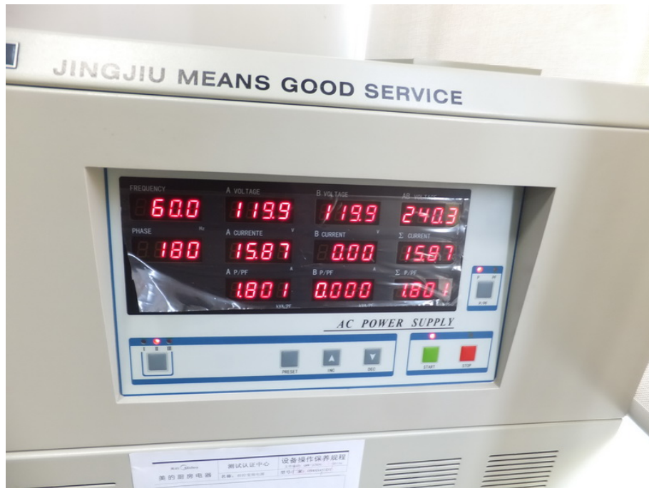
Input Power Test Set-Up (240V/60Hz)
