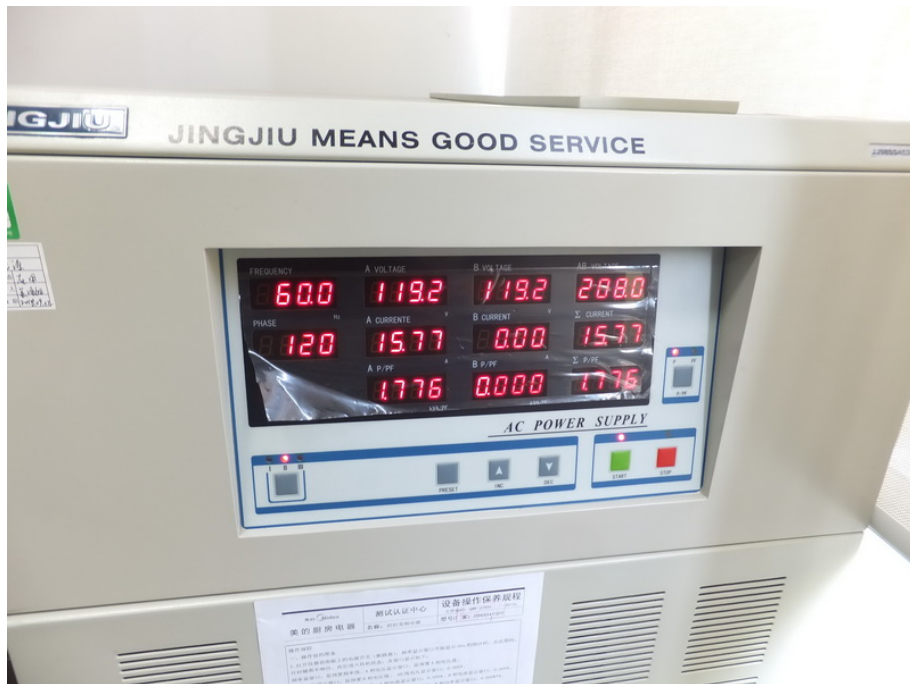
Input Power Test Set-Up (208V/60Hz)
