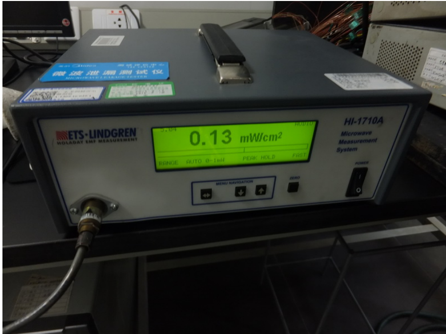
Radiation Hazard Test Set-up (208V/60Hz)
