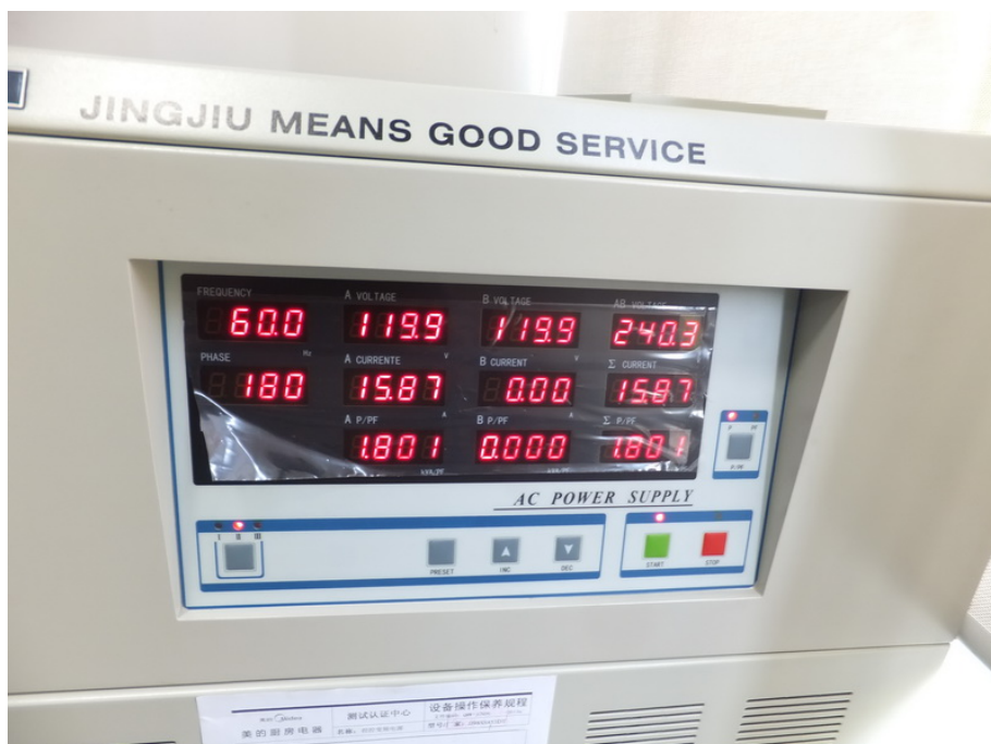
Input Power Test Set-Up (240V/60Hz)
