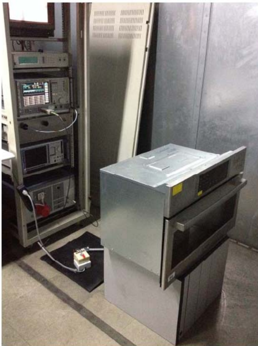
Conducted Emission Test Set-up
